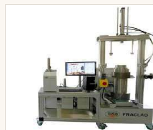
FRACLAB Hydraulic fracturing
