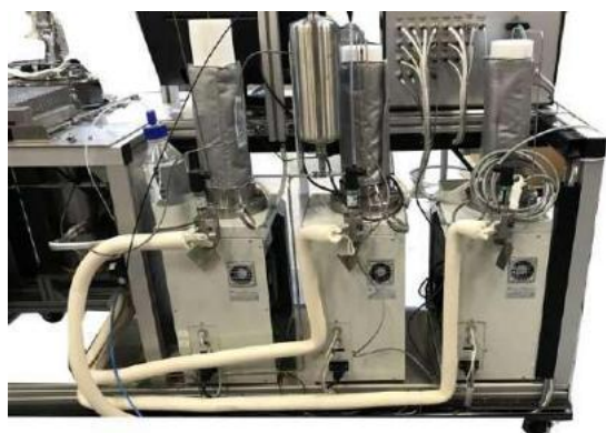
BT-series syringe pumps installed on the FRACLAB platform
