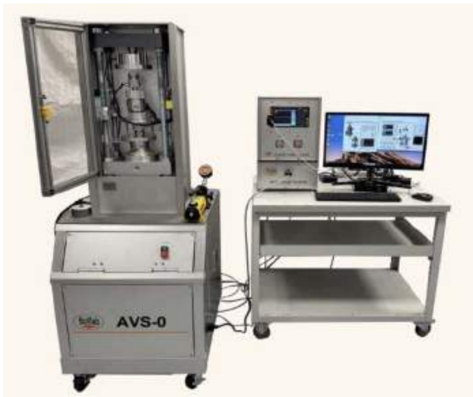
AVS-0 — 300 kN compression frame coupled to acoustic triaxial cell
