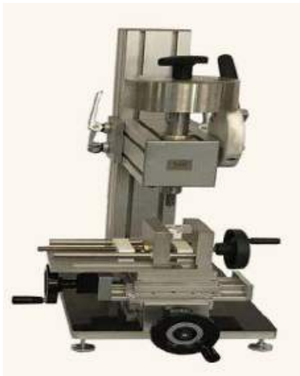
West Cerchar apparatus — fully mechanical hard-rock abrasivity tester
