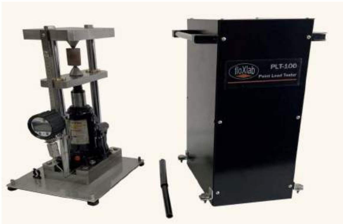
PLT100 — two-column hydraulic press with carrying case
