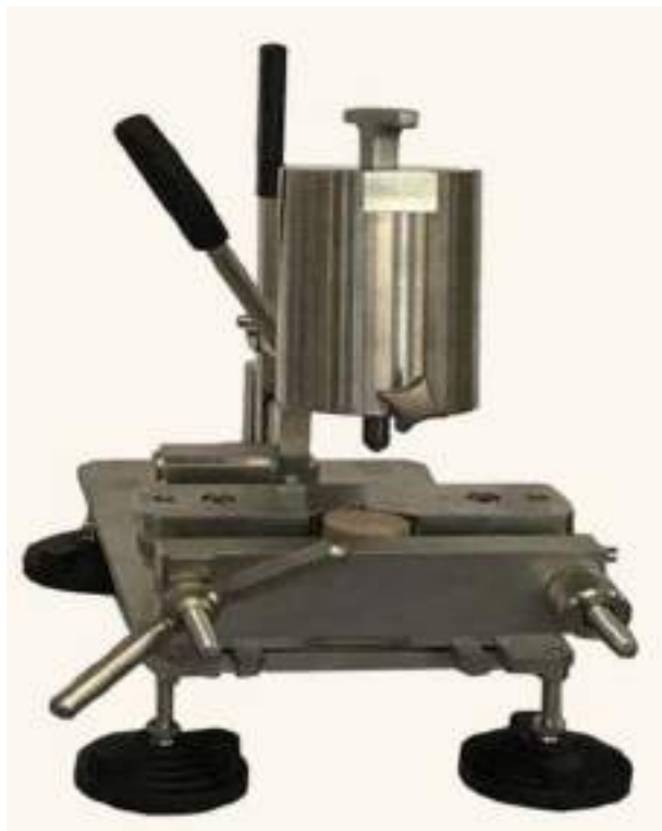
Cerchar Original — fully mechanical hard-rock abrasivity tester
