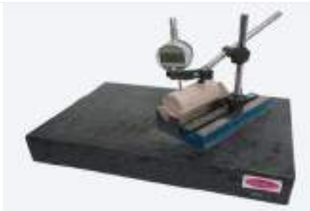
GENERAL VIEW — GRANITE BASE & DIAL INDICATOR
