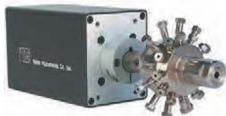
VALCO GC SELECTOR on universal actuator
